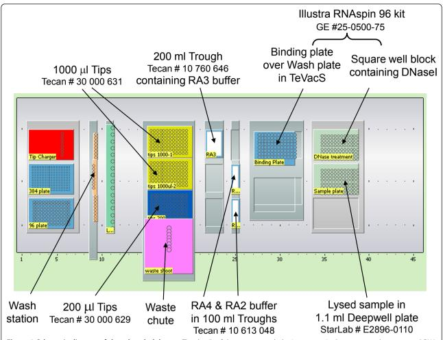
**Figure 1 Schematic diagram of the robot deck layout**. The details of the reagents and plasticware required to carry out the automated RNA extraction procedure are shown with their relative positions on the liquid handling robot deck area.
