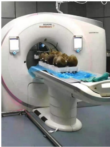
Fig. 3 CT machine scans coconut samples
