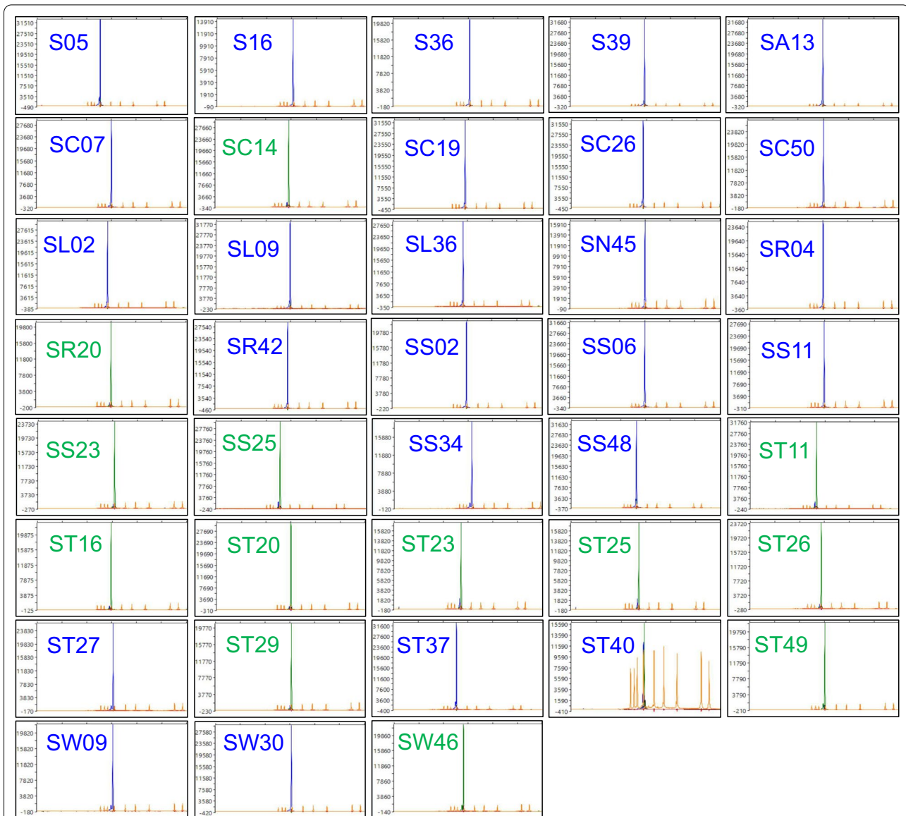
Fig. 4 The differentiating capacity of the SNaPshot assay as displayed by capillary electrophoresis of the single-spore isolates of Plasmodiophora brassicae listed in Table 2. The SNaPshot primer snpsht1-43,778 was designed against a discriminatory SNP containing an allele of A for the 5X pathotype cluster and an allele of G for the 3H pathotype cluster. Allele A fluoresces green, whereas allele G fluoresces blue. Sequencing results were visualized with Peak Scanner v1.0 (Applied Biosystems, Waltham, MA, USA). The strength of the fluorescence peak is measured against the vertical axis. The size of the SNaPshot product is measured along the x-axis against the GeneScan 120 LIZ size standards (Applied Biosystems, Waltham, MA, USA)
