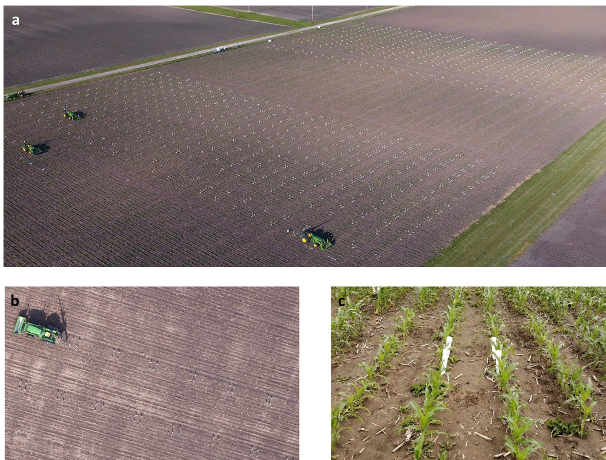
Fig. 3 Large scale minirhizotron installation in 2019, demonstrating capacity of installation with the presented method, as a aerial photograph of full experiment, b aerial photograph of portion of the experiment showing four minirhizotron tubes per subplot, c close up from ground of a single subplot showing PVC caps on tubes and normal plant growth at a later growth stage
