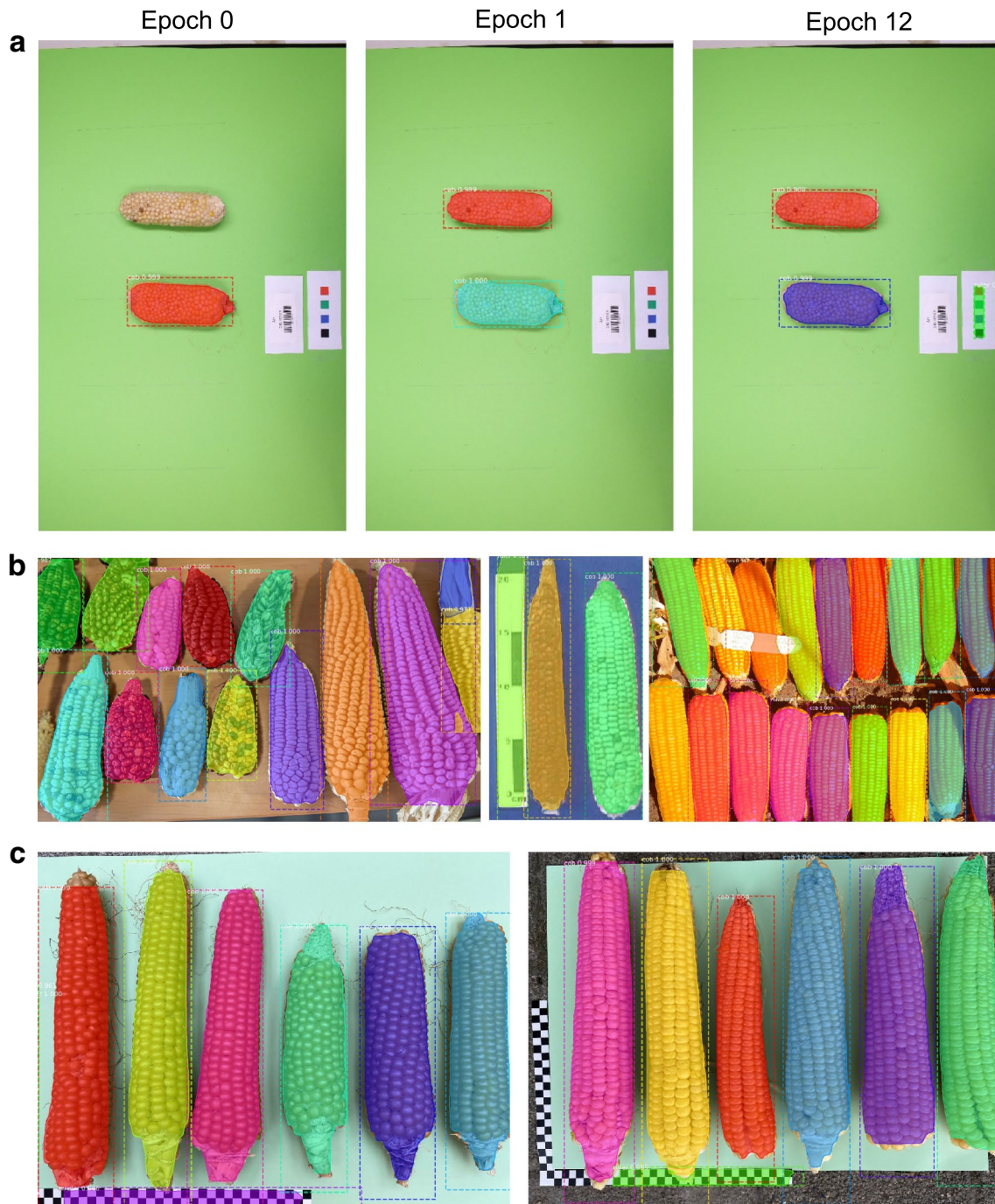
Fig. 6 Detection of cob and ruler after model updating the pretrained maize model with different image datasets. a Updating with 10 training images from ImgCross. The original maize model detected only one cob (epoch 0). After one epoch of model updating both cobs were accurately segmented and after epoch 12 the different ruler element was detected. Photo credit: K. Schmid, University of Hohenheim. b Segmentation of various genebank images after updating for 25 epochs with 20 training images from ImgDiv. Photo credits: https://hexusmedianews.com/droug-ht-is-cripling-small-farmers-in-mexico-with-consequences-for-everyone-else-photos-73b35a01e4dd (Left) https://www.ars.usda.gov/ARSUserFiles/50301000/Races_of_Maize/RoM_Paraguay_0_Book.pdf (Center) Right: CIMMYT, https://flic.kr/p/9h9X6B . All photos are available under a Creative Commons License. c Segmentation of cobs and rulers in post-harvest images of the Swiss Rheintaler Ribelmals landrace with the best model from ImgCross without updating on these images. Photo credit: Benedikt Kogler, Verein Rheintaler Ribelmals e.V., Switzerland
