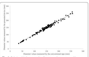
Fig. 8 Relationship between the diameter values measured by the presented device and the diameter values measured by the conventional tape
