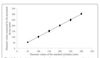
**Fig. 6** Relationship between the diameter values measured by the presented device and the diameter values of the standard cylinders
