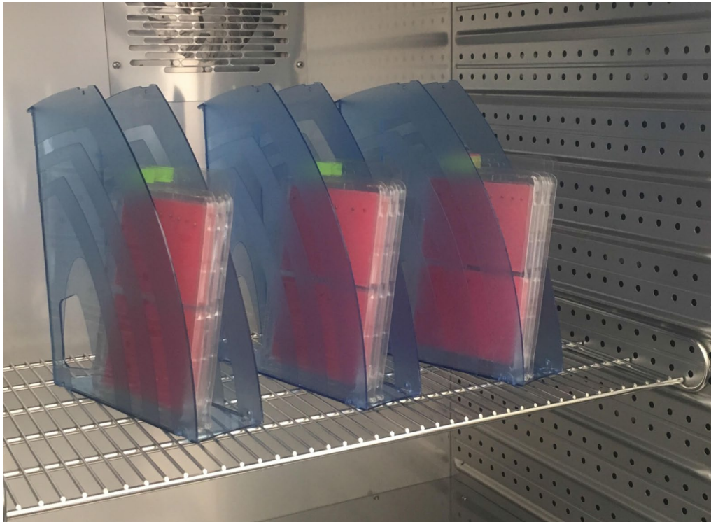
Fig. 3 Chamber with 3 groups of 3 containers installed during a single trial in the second experiment
