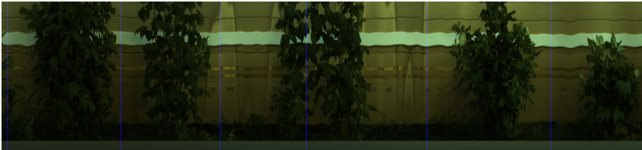
Fig. 9 Example image segmented into plant sections. Small areas of overlapping plant can be seen in centre of image that cross the lines. These are removed by excluding a 10% boundary on either side of the marked lines from the segmentation
