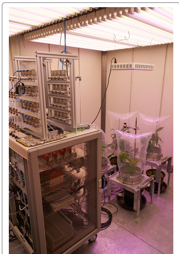
Fig. 2 Tree DEMON set-up in a climate controlled growth chamber. Left side BVOC sampler unit on top of a 19 in. rack with mass flow controllers, data acquisition unit, control pc and infrared gas analyzers (not visible, located behind the rack). Right side four plant chamber systems with built-in trees. Top right side LED panel for increasing light intensity received by the plants
